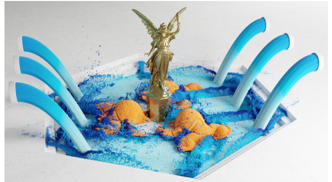
Fig. 14. Multi-resolution two-phase simulation of high- and low-viscosity fluids. Six emitters pour up to 5 million fluid particles into a pool with a static rigid body (Stanford Lucy) and three highly viscous Stanford Armadillos. The 90 thousand particles of the viscous material have a 2.5 times larger radius than the fluid particles.
